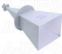
LB-62-25-C2-SF Standard Gain Horn Antenna 12.4-18GHz 25dB Gain SMA Female
